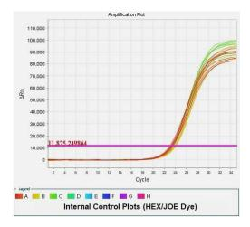
Internal control amplification plots must be seen in all wells except NTC and has been labelled with HEX (JOE) dye. The CT value of internal controls should be  $22 \le X \le 26$ .
