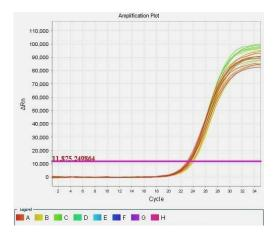
Internal control amplification plots must be seen in all wells except NTC and has been labelled with CY5 dye. The CT value of internal controls should be  $22 \le X \le 26$ .
