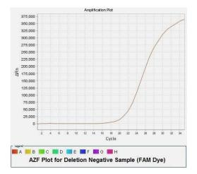
Amplification plots of AZF's can be analysed by FAM dye. The CT value should be between **18**  $\leq$  **CT**  $\leq$  **25**. These values are optimised according to the MN NucleoSpin <sup>®</sup> Blood DNA Isolation Kit. CT values could be vary ±2/3 cycle according to the DNA isolation protocol.
