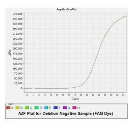
Amplification plots of AZF regions can be analysed by FAM, HEX/JOE and TEXAS RED dyes (Please check table -1). The CT value should be between **18 ≤ CT ≤ 25**. These values are optimised according to the MN NucleoSpin <sup>®</sup> Blood DNA Isolation Ktt. CT values could be vary  $\pm 2/3$  cycle according to the DNA isolation protocol.
